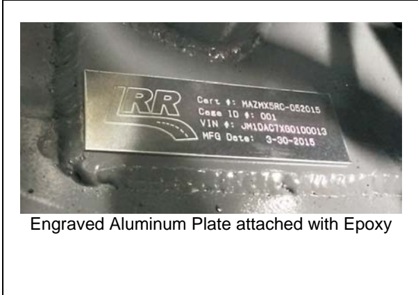
PHOTO 12 DETAIL OF IDENTIFICATION PLATE
