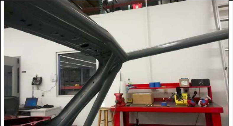
PHOTO 9 ATTACHMENT TO FRONT SUSPENSION
